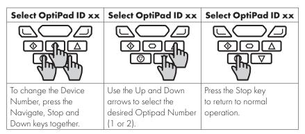
NOTE Once the User has set the Optipad as Device Number 2, OptiTools software cannot be used on the same drive network. The Optipad Device Address should only be changed to 2 if 2 Optipad units are connected on a network. An Optipad with Device Number 1 must always be present for the network to function correctly.
