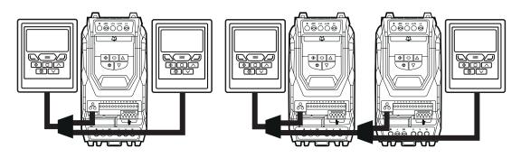
Different drive models can be used on the same Optipad network provided a unique communications address is assigned to each. NOTE Cannot be used with Master – Slave or Cascade Control
